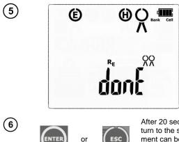
When the **donE** is displayed on the screen, the clamp calibration procedure is completed.
