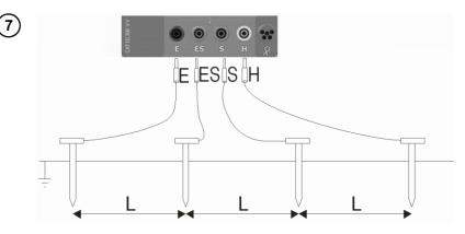
Connect the four aligned and equally spaced electrodes, which are driven into the ground, to the meter, and do so In accordance with the diagram above: Connect the current electrode driven into ground to the **H** socket of the meter, Connect the voltage electrode driven into ground to the **S** socket of the meter, Connect the voltage electrode driven into ground to the **ES** socket of the meter, Connect the current electrode driven into ground to the **ES** socket of the meter.
