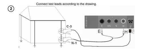
Connect the transmission clamp to sockets  ${\bf H}$  and  ${\bf E},$  while the measurements clamp should be connected to the clamp socket  ${\bf X}.$
