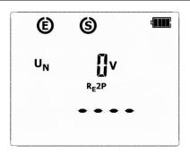
In R<sub>E</sub>2P, R<sub>E</sub>3P, R<sub>E</sub>4P, R<sub>E</sub>3P+C, R<sub>CONT</sub> and  $\rho$  modes, before starting the measurement with the **START** button, MRU-30 is monitoring the voltage present on the measurement points (between **E** and other sockets). The value of the interfering voltage is displayed on screen.
