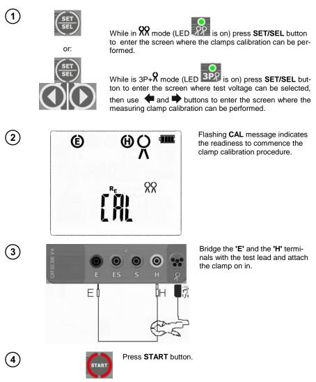
The meter has determined the correction factor for connected clamp. The factor is saved in the memory also when the power supply of the meter is off until the following successful calibration of the clamp has been performed.
